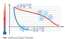
with blast freezer: avoids the formation of macrocrystals, assisting the formation of microcrystals
